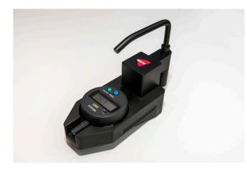
DELTA's Marking Thickness Gauge is a digital devise for measuring the thickness of pavement markings dry, after application. The Marking Thickness Gauge is very easy to operate and comes in a sturdy construction and ergonomic design. The Marking Thickness Gauge can measure markings within the measurement range of -12.7 mm to +12.7 mm / -0.5 inch to +0.5 inch. The digital display provides reliable measurement results in seconds.
